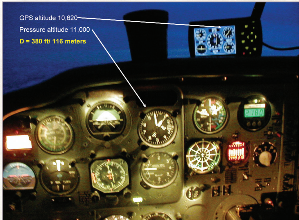
Figure 3: Approaching SEDAR on flight from Honolulu. Note difference D between pressure altitude and GPS altitude, consistent with 700 mb pressure chart. GPS altitude is analogous to radar altitude over the sea. Altimeter set at 29.92" displays pressure altitude.
